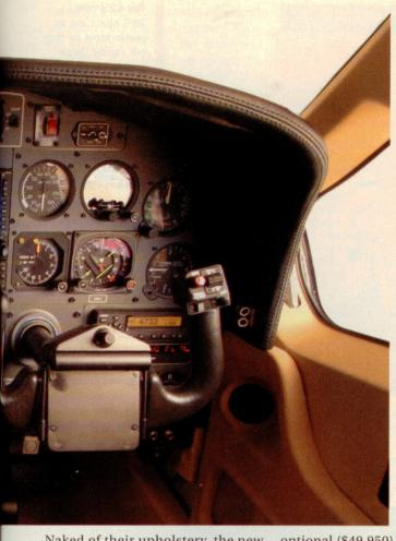
A Honeywell EFIS package, a pair of Garmin 530s, and Honeywell's **Integrated Hazard Awareness System** (IHAS) fill out the standard panel. Trim position indicators take up prime real estate on the center pedestal, for good reason. Torque at high power settings requires hefty amounts of right-rudder trim for takeoff.
